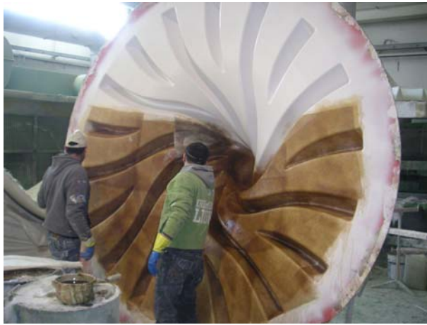
Impeller dia. 2700 under construction
