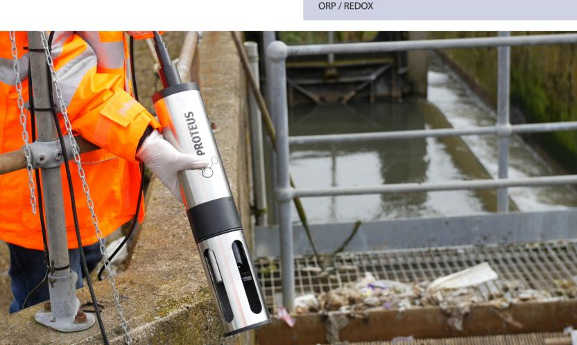
**Self cleaning:** As it is essential that optical sensors have a cleaning mechanism, the Proteus is also supplied with an integral wiper which cleans all of the Proteus' sensors before every measurement cycle.
